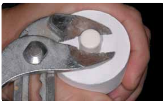
The Alox plunger is already very clean if it is removed with tongs from the investment material. Check the cleanness and blast with Al_2O_3 , if required.
