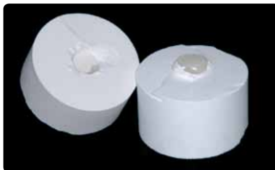
Separate the investment ring using a separating disk.
