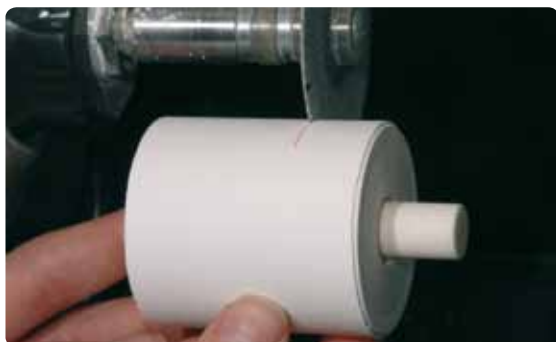
Separate the investment ring using a separating disk.
