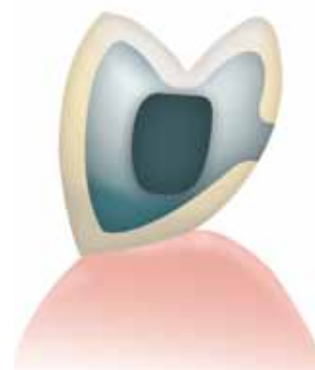
Double the height of the connector with single width = eightfold stability
